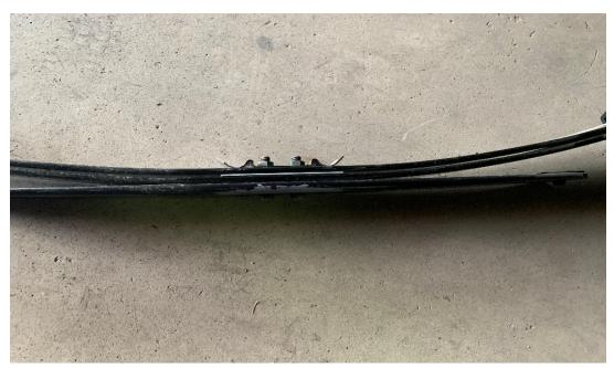
Using a c-clamp to hold the leaf springs together, carefully remove bolts and flip them around. See pic below for details.
