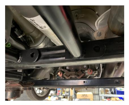
Step 5. Re install the (4) drive shaft bolts and torque down to 83ftlbs. Your DS Loop is now ready for use.
